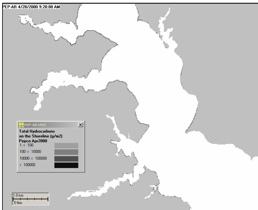
Figure 9. Total hydrocarbons (g/m 2 ) on the shore (no shoreline cleanup simulated) after 21 days (view 2).
